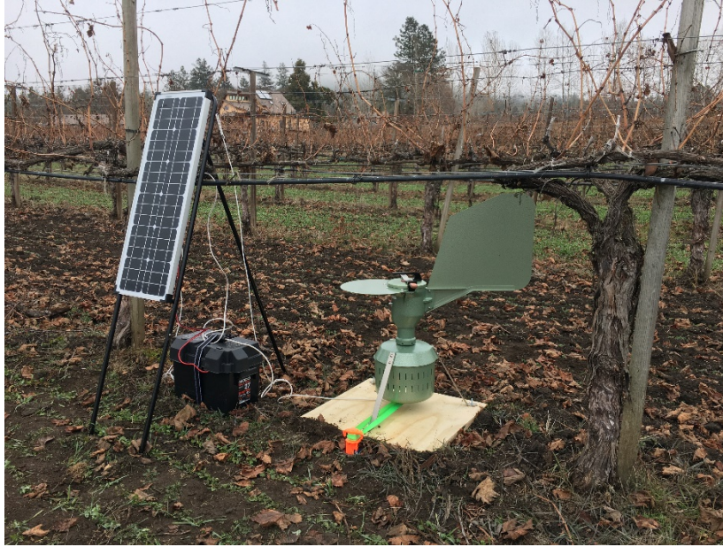
Figure 3: A Burkard volumetric spore trap set up in a vineyard in the Applegate Valley.
