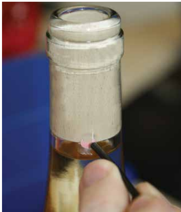
Winemakers use NomaSense technology to measure oxygen pickup inside tanks, hoses, pumps and bottles (above).
